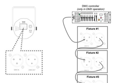
In order to use this fixture in a DMX or master/slave operation, you must daisy chain, using DMX cables to link from one fixture to another.
